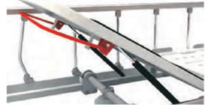
Lifting Rod, located at head side of backrest to allow one hand lifting of back board through two pneumatic cylinders.
